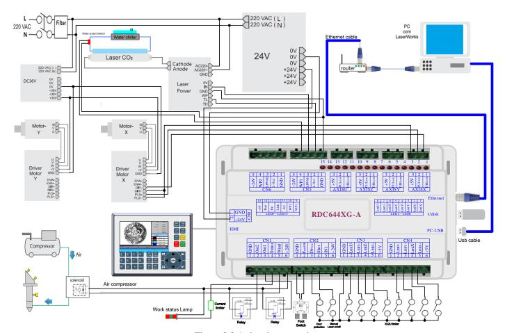
Figure 3.3-1 electric connection
